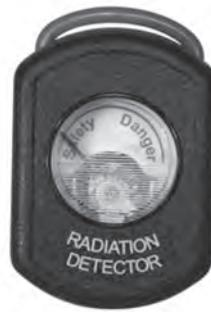
The detector is held next to the microwave oven to see if any microwave radiation is leaking to the surroundings.
